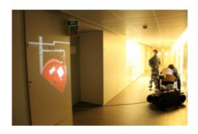
Your task in this project will start out in the lab: You will use an RGBD camera to identify a wall / flat surface. Then, you will use an LED-based Video Projector to project an imager onto that surface. Finally, you will install this on the SPOT robot
